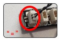
Connect the AAA Battery Pack to 4-Port Expansion Boards.
