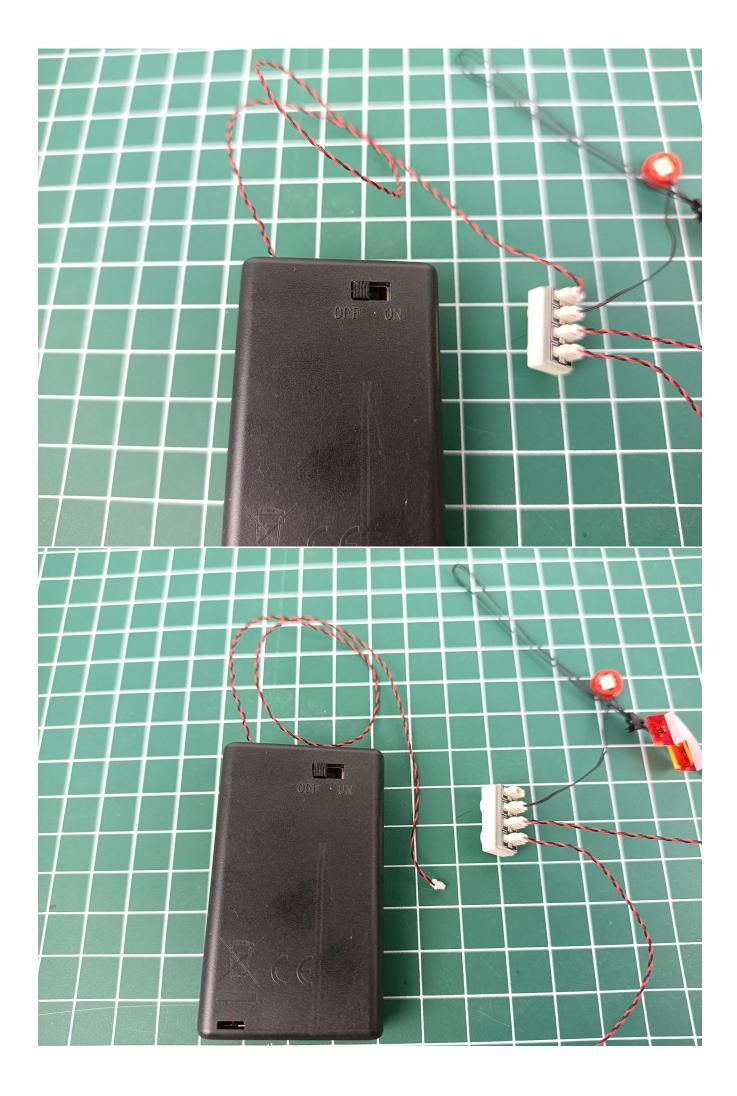
Take out the USB power cord and connect it to 4-Port Expansion Boards.
